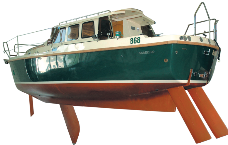
View of the under water part of the HABER 800C4 yacht with all centerboards dropped.
